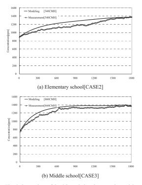
Fig. 6. Comparison of the  $CO_2$  variations between the modeling and the experimental results.
